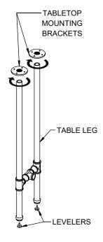
PLACE THE FIRST LEG DOWN ON THE GROUND AND THREAD ON THE SECOND LEG BY ROTATING CLOCKWISE UNTIL TIGHT.
