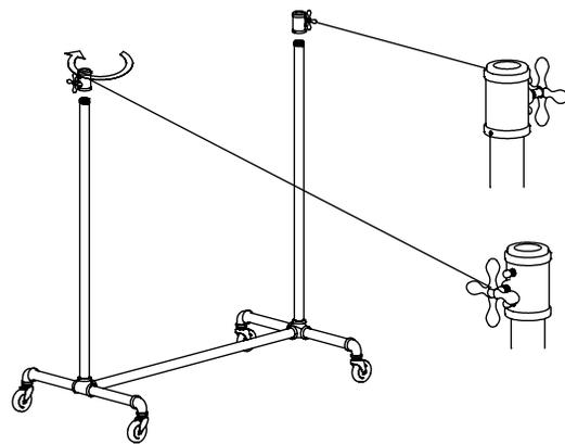
BY HAND, SCREW ADJUSTABLE CONNECTOR TO BOTTOM UPRIGHTS.
