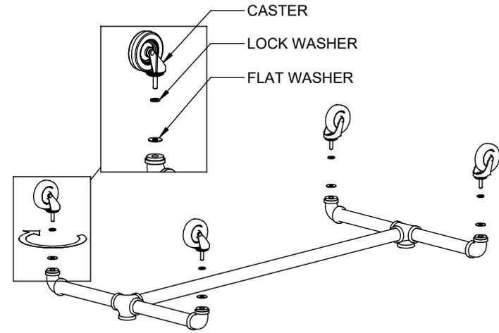
SCREW IN THE CASTERS TO THE BASE AS SHOWN USING PROVIDED WRENCH.
