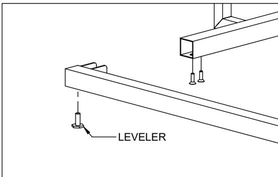
IF THE LEVELERS ARE NOT ALREADY INSTALLED, INSTALL THEM ONTO THE LOWER CROSS BARS. SECURE THE LOWER CROSS BARS TO THE ASSEMBLY FROM STEP 1 WITH THE REMAINING COUNTERSUNK SCREWS.
