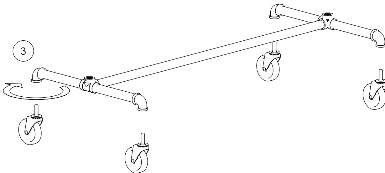
3 SCREW IN THE CASTERS AS SHOWN USING PROVIDED WRENCH
