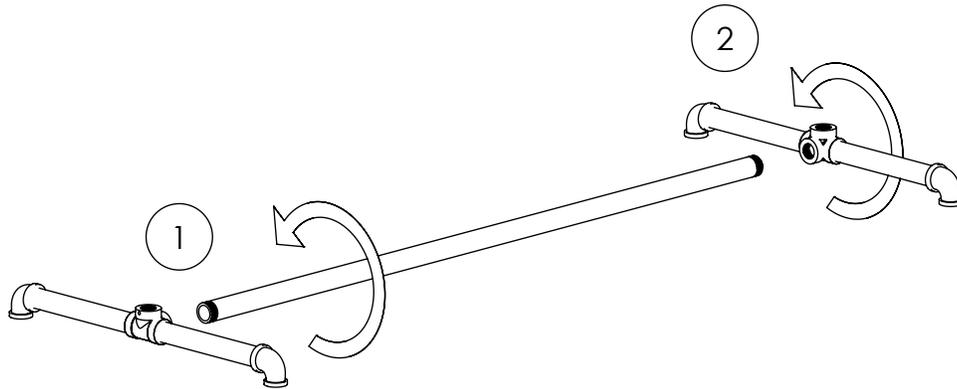
1 BY HAND, SCREW IN THE CROSSBAR TO FOOT AS SHOWN. TIGHTEN FULLY.
