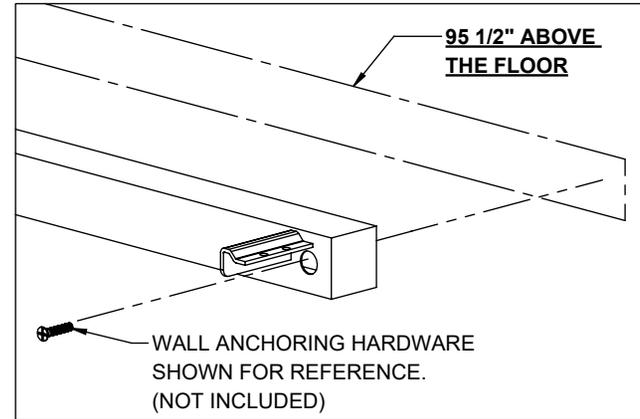
LEVEL AND MOUNT THE TOP CROSS BAR TO THE DESIRED WALL AS SHOWN WITH APPROPRIATE WALL MOUNTING HARDWARE.
